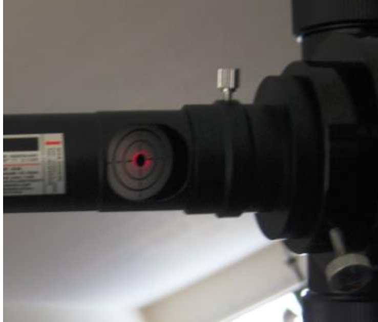
Figure 2: The primary mirror is perfectly collimated by laser collimator.
