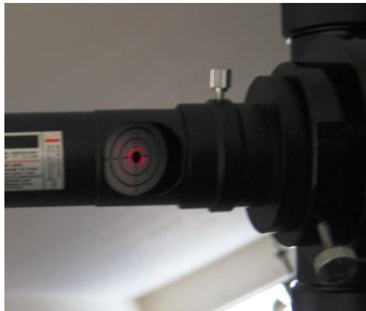
Figure 4: The primary mirror is perfectly collimated by laser collimator.
