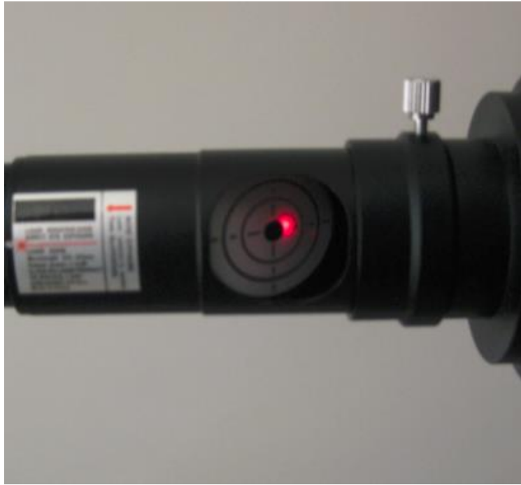
Figure 3: The primary mirror is not yet collimated.
