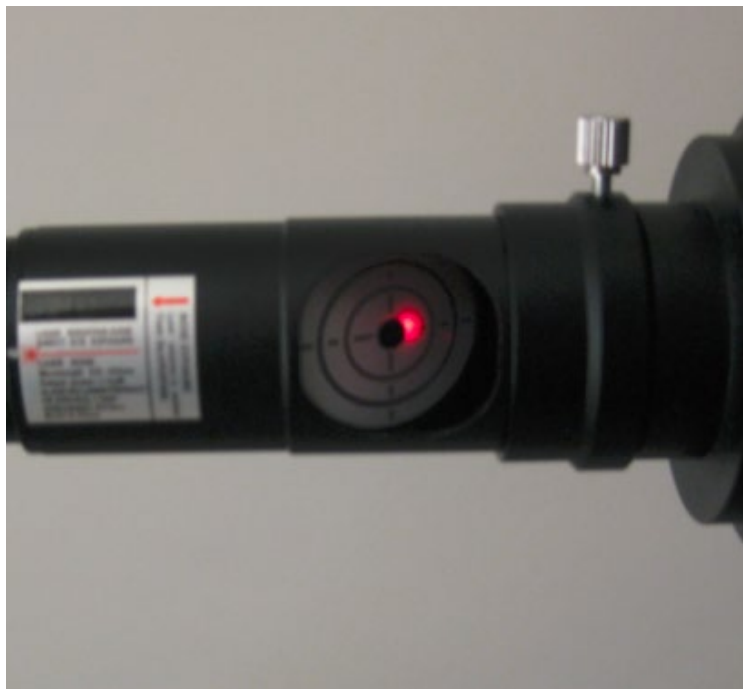
Figure 10: The primary mirror is not yet collimated.
