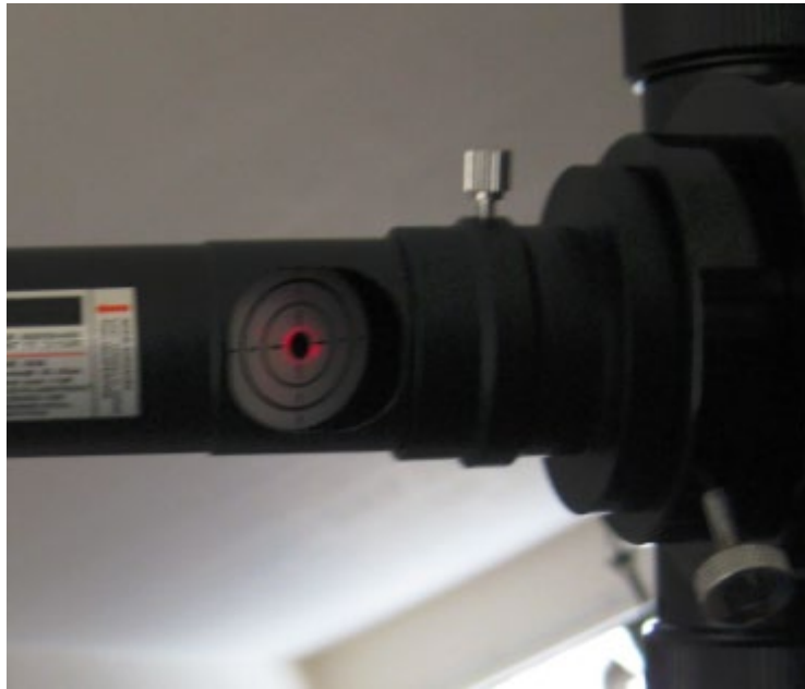
Figure 9: The primary mirror is collimated by laser collimator.
