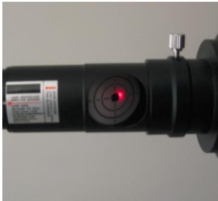
Figure 10: The primary mirror is not yet collimated.
