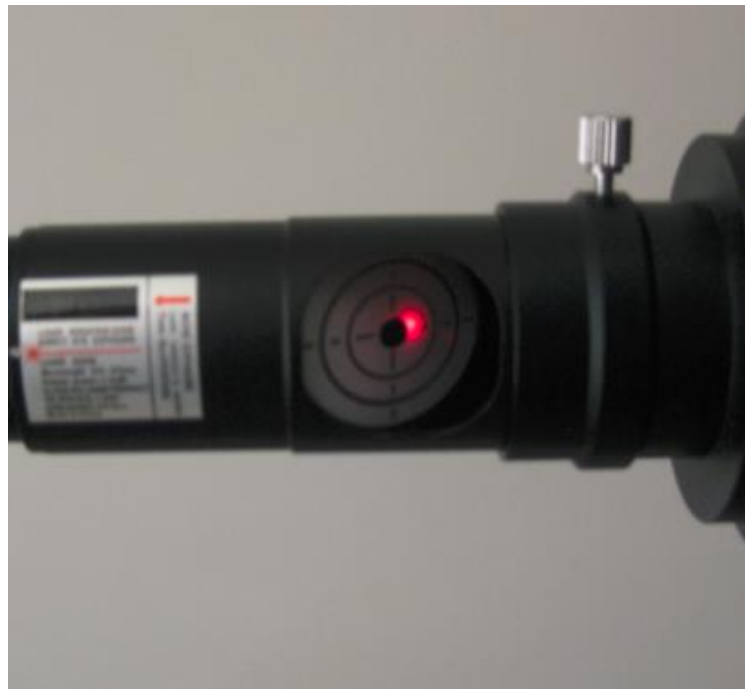
The primary mirror is not yet collimated.
