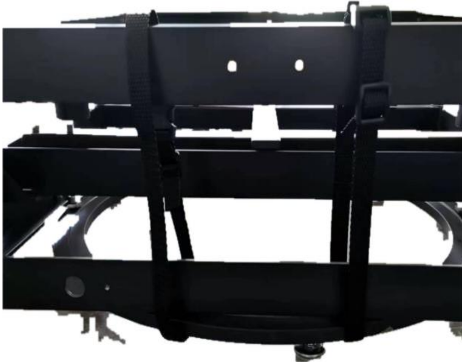
Lock the mirror box to the rocker with nylon strips.
