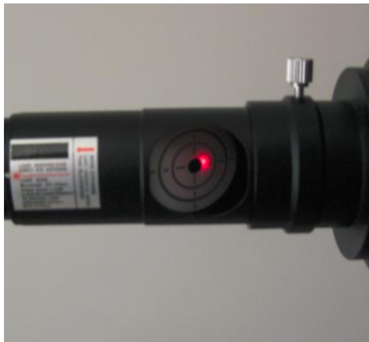
The primary mirror is not yet collimated.
