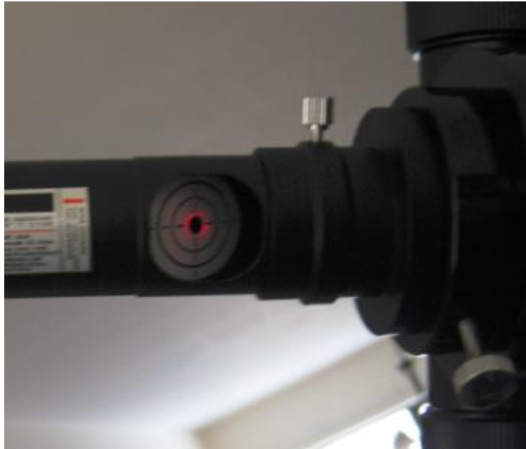
The primary mirror is fully collimated by laser collimator.
