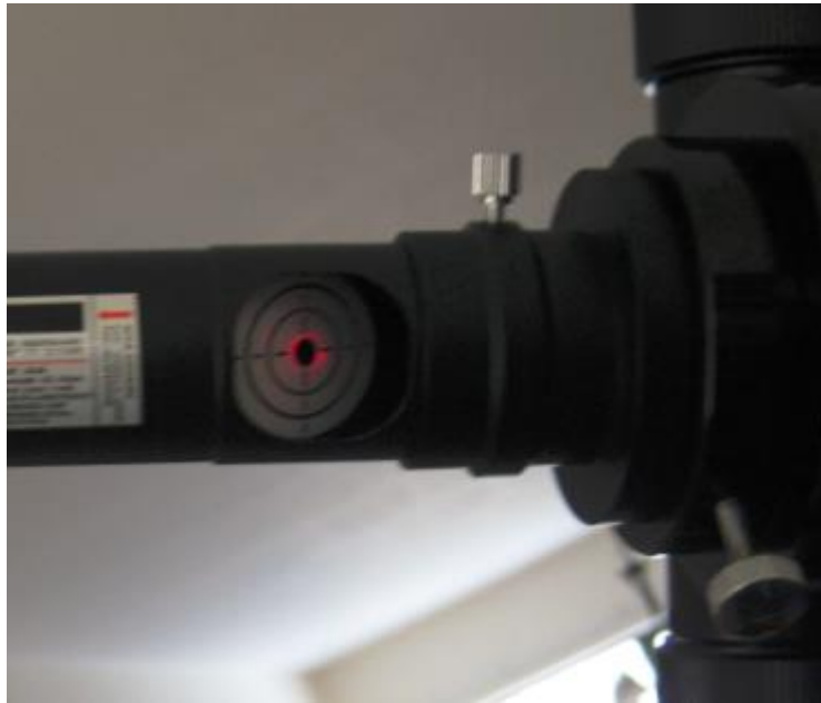
The primary mirror is collimated by laser collimator.
