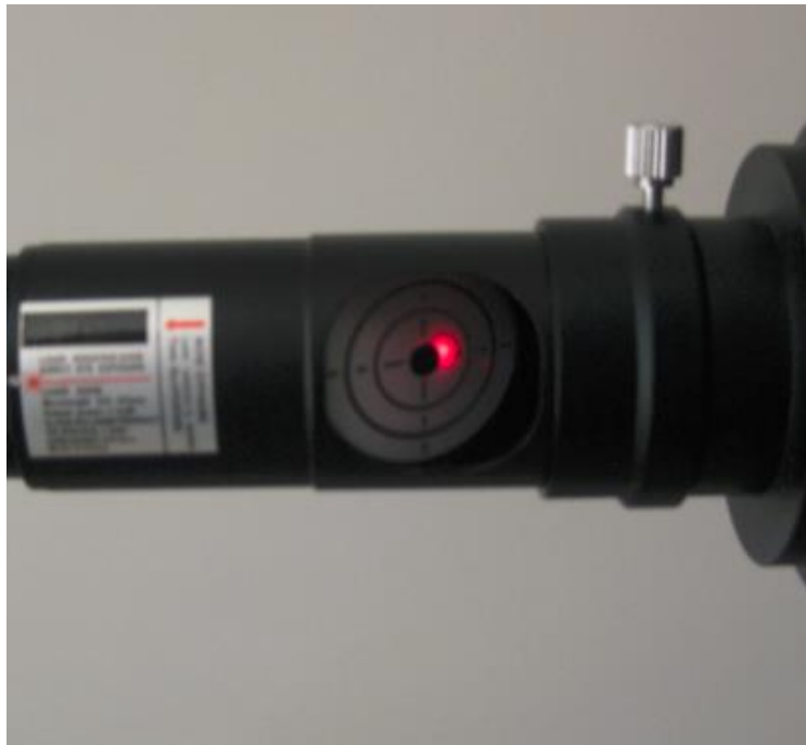
The primary mirror is not yet collimated.
