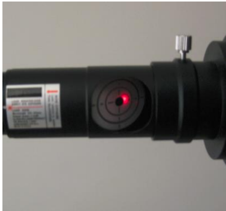
The primary mirror is not yet collimated.
