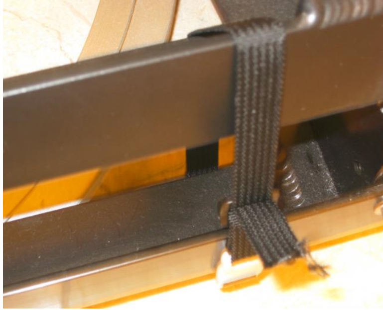
Lock the mirror box to the rocker with nylon strips.
