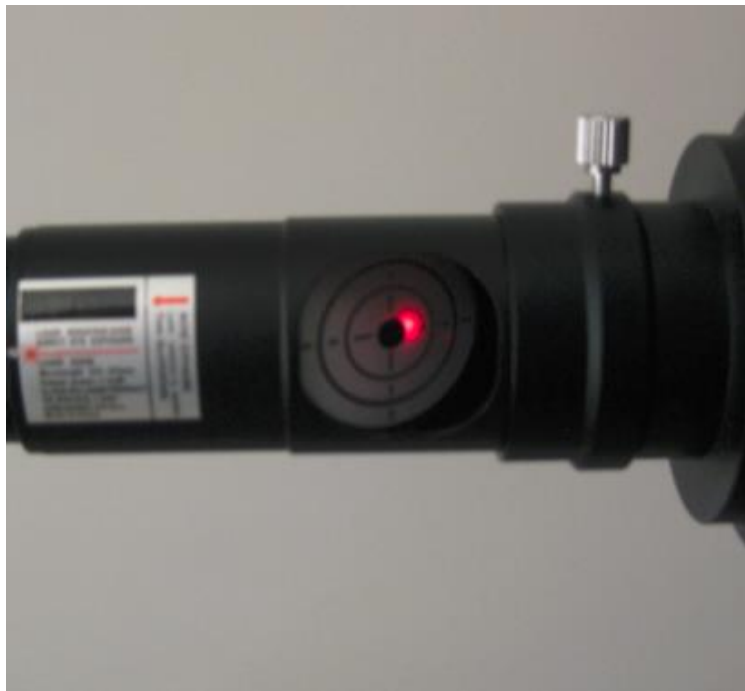
The primary mirror is not yet collimated.
