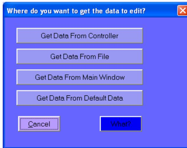
The data that populates the windows in the Edit Parameters Tool will come from whichever of these sources you pick. **Most of the time you will use the “Get Data From Controller” option.** Select this option as we go through initially setting up your controller.
